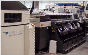
Philips Assembléon high-speed SMT line places 60,000 parts per hour and handles parts as small as 01005.
