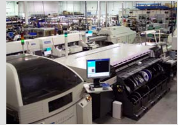
With both high-speed and high-mix lines, we produce PCBs with SMT 01005, BGA and \mu BGA components.
