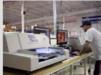
We assure quality through ISO processes and equipment such as automated optical inspection (AOI).
