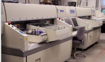
MYDATA dual SMT line offers quick change-over for small runs & online component testing for high quality.
