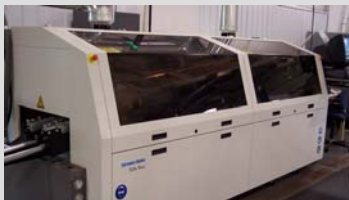
Vitronics Soltec Delta lead-free wave solder with computer control allows us to store and quickly set up the best process for each board.
